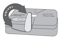
2. Rotate the stand on the bottom of both speakers. Then place both speakers on a level surface.
